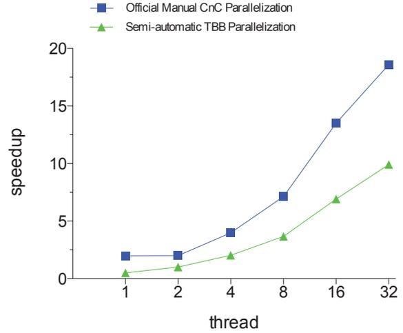
Figure 10: FaceDetection speedups with different threads
