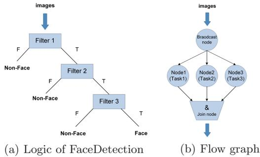
Figure 9: FaceDetection logic and flow graph
