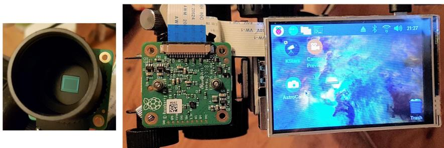
Figure 1: Camera Sensor with C-Mount Telescope Adapter and Hubble Pi Board
