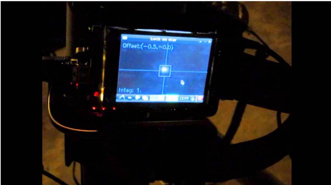
Figure 8: Python Based Raspberry Pi AutoGuider by [Samson Yang](#)
